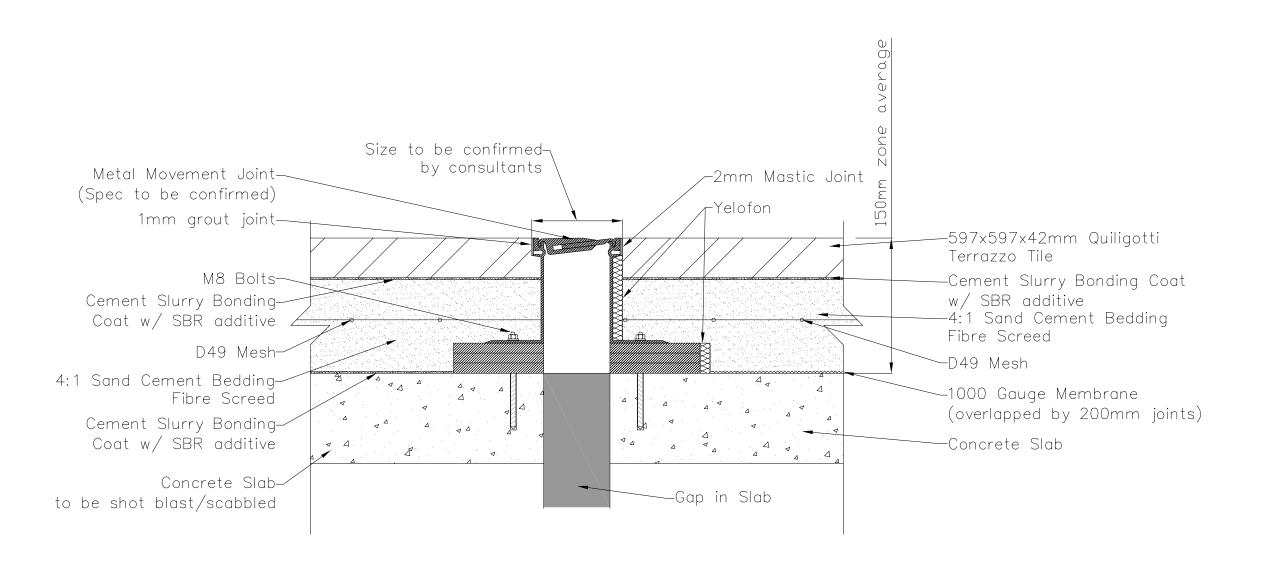
TYPICAL STRUCTURAL MOVEMENT JOINT DETAIL
